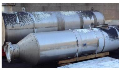
stage, and on the other, because material in this condition is unsuitable for reuse, it might deteriorate (by corrosion). The only option then is to anneal at a temperature of 900 °C which renders the formed carbides resoluble, followed by rapid cooling. In practice, however, this tends to be unfeasible.
