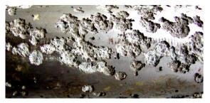
**Crevice corrosion** is another type of corrosion that can occur due to the presence of contaminations on a stainless steel surface. Inorganic contaminants are salts that may be present in either a dissolved or undissolved form. In an undissolved form, thus in the form of a solid contamination, the problem will be similar to the under-deposit corrosion referred to. In a dissolved form, the salts may lead to corrosion.
