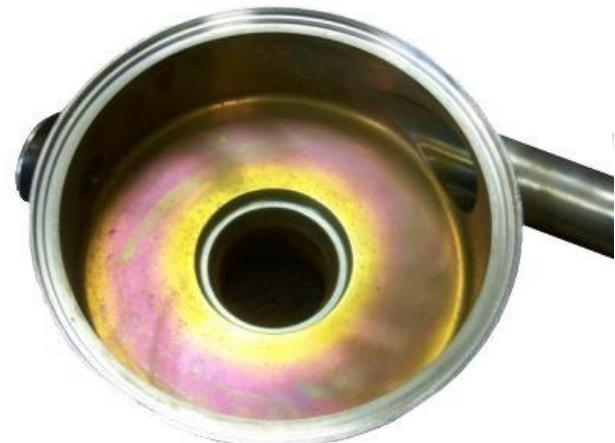
*Pump casing with rouging before treatment*
