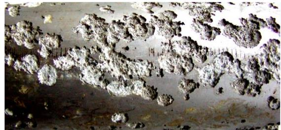
**Crevice corrosion** is another type of corrosion that can occur due to the presence of contaminations on a stainless steel surface. Inorganic contaminants are salts that may be present in either a dissolved or undissolved form. In an undissolved form, thus in the form of a solid contamination, the problem will be similar to the under-deposit corrosion referred to. In a dissolved form, the salts may lead to corrosion.
