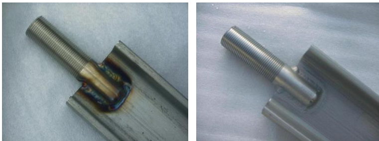
Left: stainless steel with heat tint. Right: the heat tint has been removed by pickling. The corrosion resistance has been fully renewed
